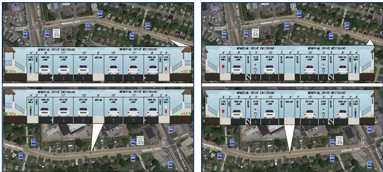
Figure 22: Before (left) & After (right) the Condition of the Road Diet Project Along Memorial Drive
